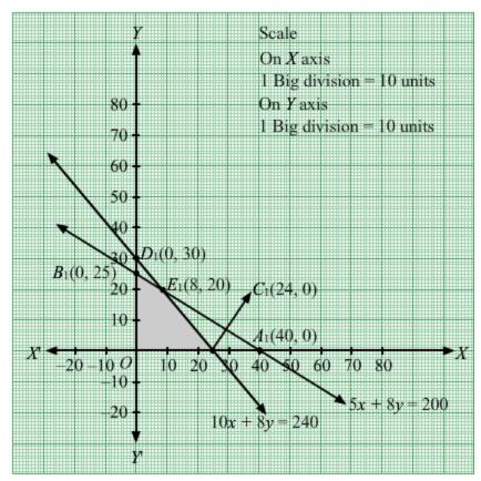
The corner points of the feasible region are O(0, 0),  $B_1(0, 25)$ ,  $E_1(8, 20)$ ,  $C_1(24, 0)$ . The values of Z at these corner points are as follows.
